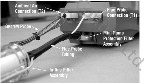
WARNING: - Ensure the 'K' type thermocouple probes are inserted into the sockets correctly (see page 7). The plugs are polarity marked and forcing the plug into the socket the wrong way may result in damage to the instrument.
