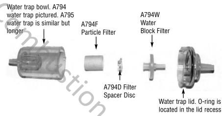
Open the water trap and look at the A794F particle filter. The filter will typically get dirty from the inside first. If the filter is dark on the inside a replacement filter should be installed.
